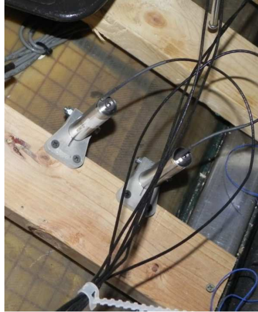
Figure 6-9 Static Load Test LVDTs
