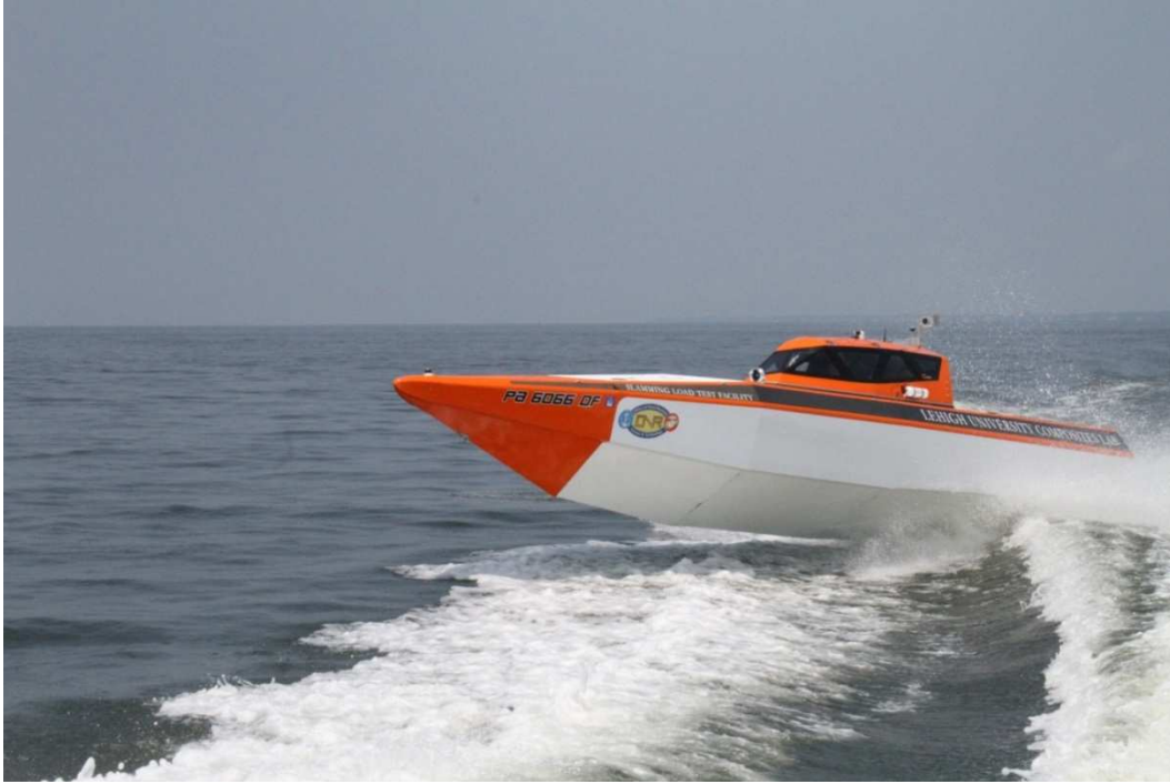
Figure 7-2: Numerette slamming test boat
