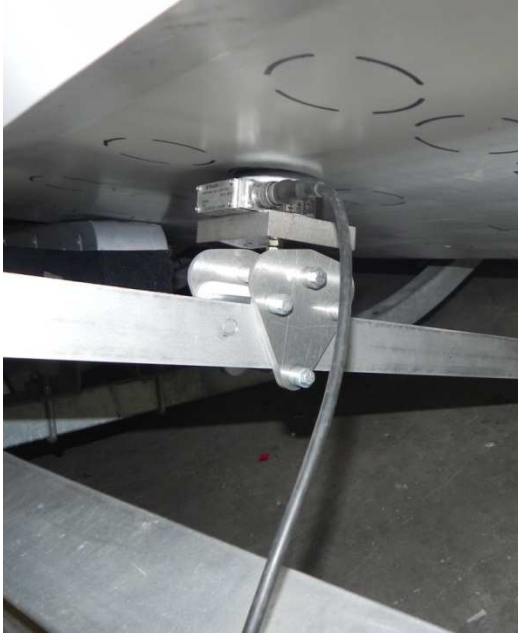
Figure 6-8 Static load test fixture
