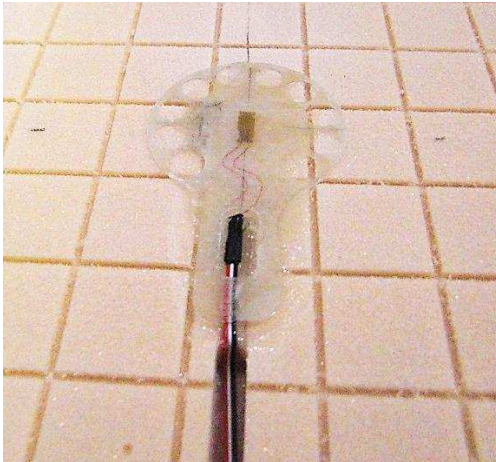
Figure 6-3: Strain gage paddles bonded to PVC foam core
